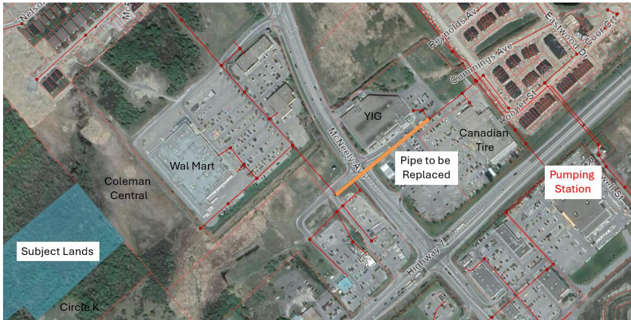
Figure 13 – Area of Downstream Sanitary Capacity
