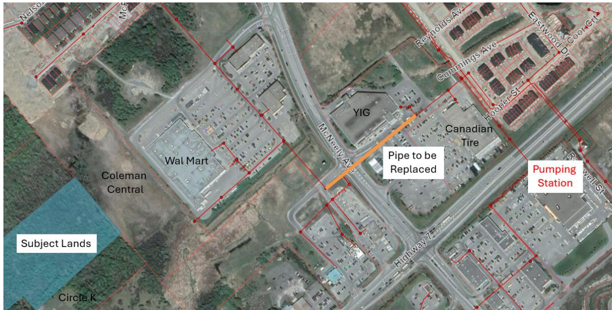
Figure 13 – Area of Downstream Sanitary Capacity
