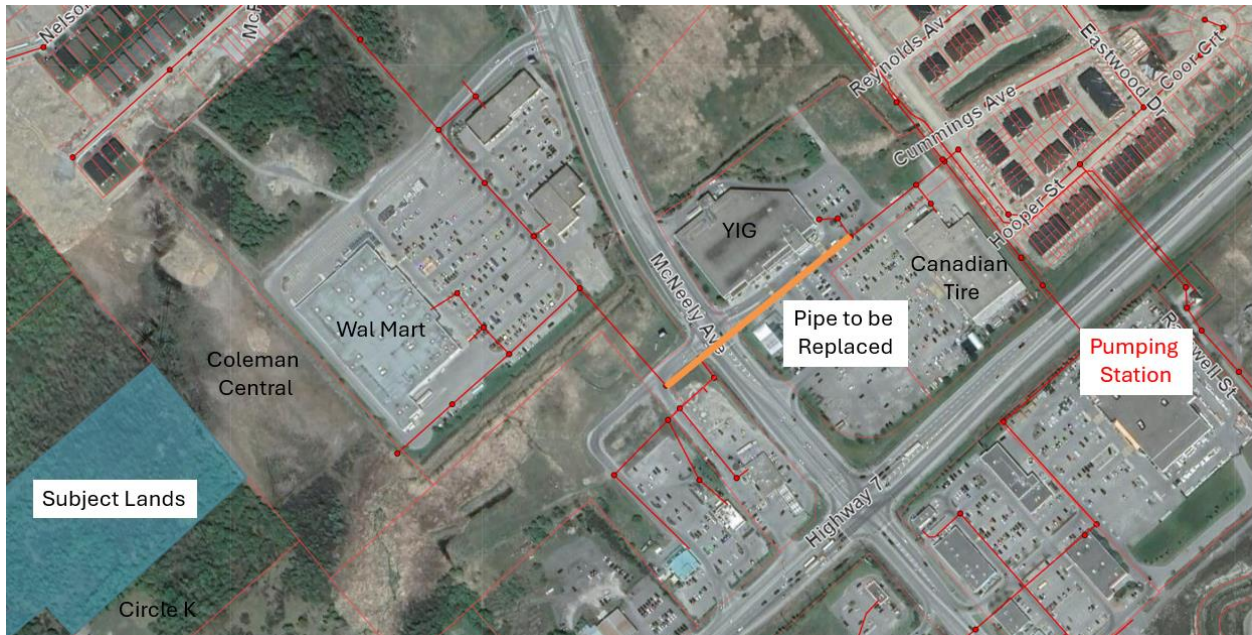
Figure 13 – Area of Downstream Sanitary Capacity
