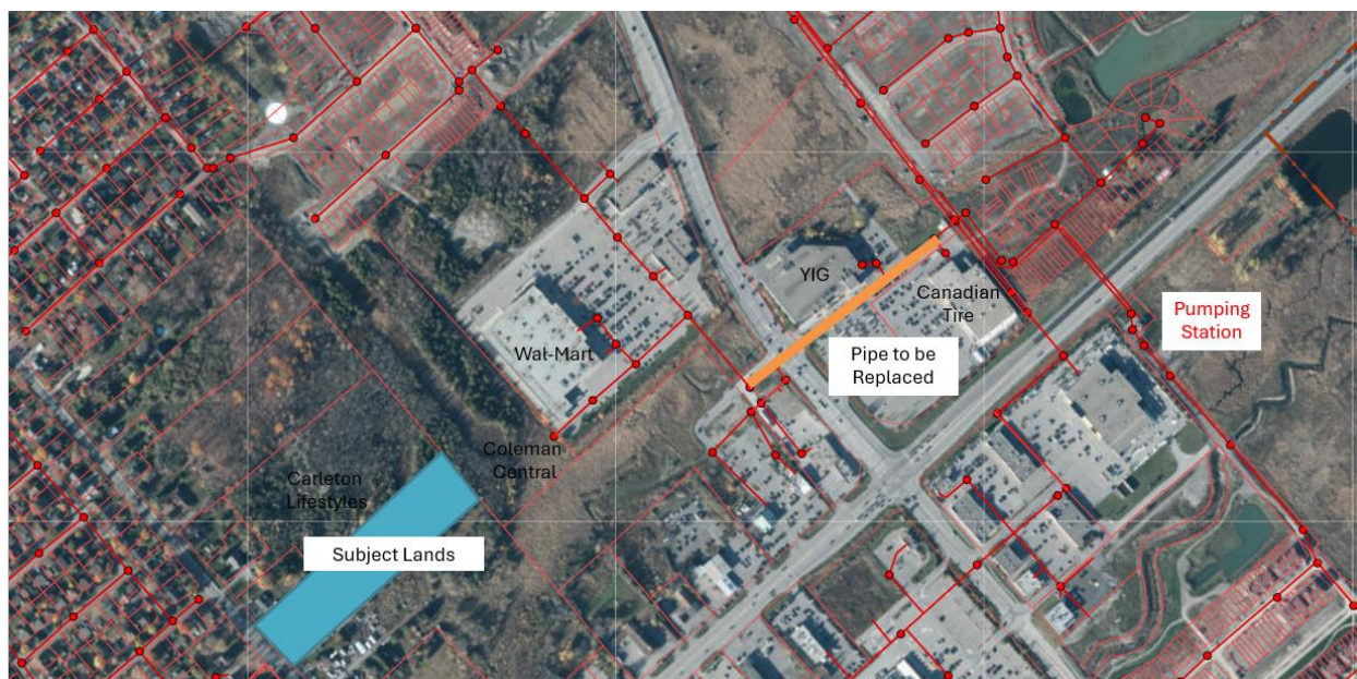
Figure 13 – Area of Downstream Sanitary Capacity
