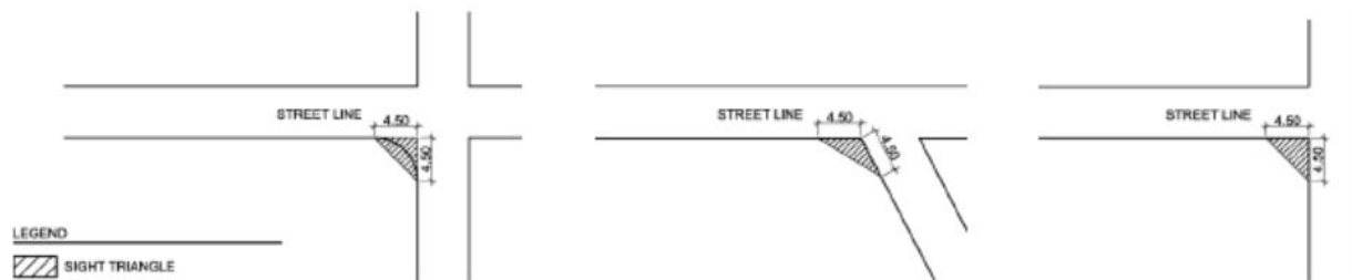
Figure 3.13. Calculation of a Sight Triangle
